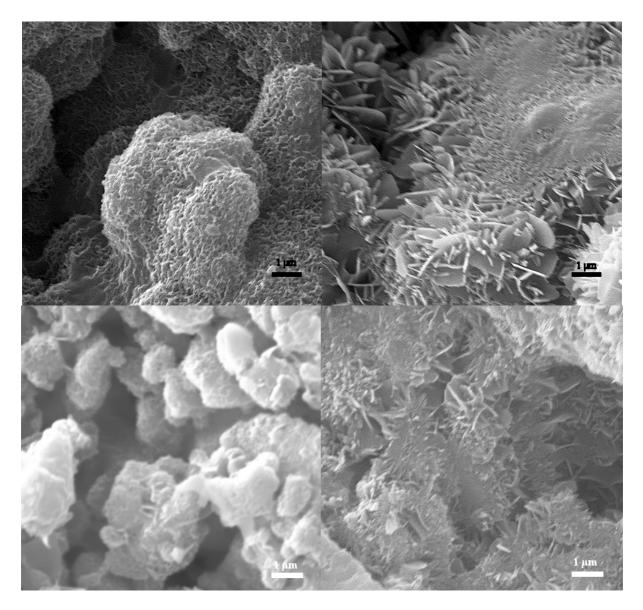
Figure 2. SEM microphotographs of as-prepared and fracture surfaces of unmodified (I) and modified (V) cements after setting and immersion in SBF for 192 h (10000 X). Upper left: I external surface; Upper right: I fracture surface; Lower left: V external surface; Lower right: V fracture surface.
