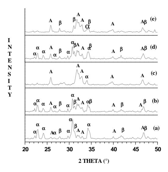
Figure 1. X-RD patterns of cements I and V at different stages of setting.(a): I unreacted powder; (b): I after mixing and conditioning 1 h at 100 % R.H.; (c): (b) after immersion in SBF at 36,5 °C for 192 h; (d): V after mixing and conditioning 1 h at 100 % R.H.; (e): (d) after immersion in SBF at 36,5 °C for 192 h.  $\alpha$ :  $\alpha$ -TCP;  $\beta$ :  $\beta$ -TCP; A: hydroxyapatite.
